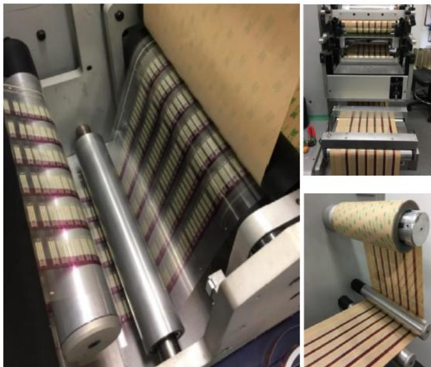
Figure 3: Biosensor manufacture at the Australian National Fabrication Facility
