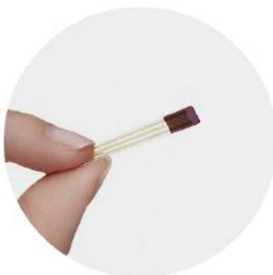
Figure 14: The Saliva Glucose Biosensor Strip Biosensor
